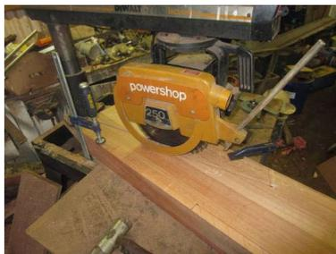
A band saw would have been a better tool for this job, but I just have the radial arm and a hand held 'Skil' saw, so after cutting the end off at 60 degrees I simply clamped the block down on the table, very accurately set the blade up on the correct side of the line and worked back and forth dropping the blade by a small amount each time. I couldn't get all the way through the wood, so I had to turn it over and do the rest from the other side. It's always a
