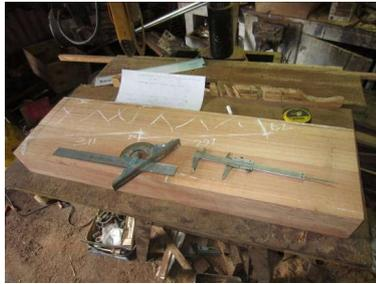
The block was a few millimetres too wide and there was a slight slope on the far side, so this gave me the opportunity to correct both. For my measurements at the Mill, I was working from both edges, so the new piece had to be exactly the same! The radial arm saw made heavy weather of the cut which I had to do in six passes; the wood's that hard! The advantage was that I could check for squareness as
