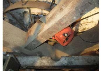
Would I have to loosen off all the bolts and move the pit-wheel forward? That would also mean un-meshing the pinions to get them out of the way. The pinion for the Vitruvian Mill is wedged, but it still needs a jack in place to lower it with. I have never touched the pinion which drives the pulley to drive the rest of the Mill House!
