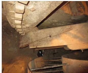
The only other plan I could think of was to cut out a section of the cant, equivalent to the depth and width of the original slot, as long as the width of the arm, and tap the off-cut across into that. I removed most of the wood by drilling three holes with the same flat bit that I'd used earlier. I knew the bolt and square nut would also be in the way, so that had to be removed too, along with one cog.
