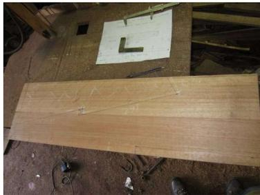
I marked out each side as I had in the Mill, starting at the same place on each side, allowing this time for the gap for the wedges. I was delighted when I drew across with a square from one side to the other, that the lines met exactly!
